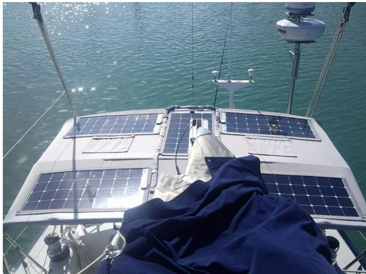
Note that the Velcro is both sewn and glued to the panel. Also note that in this case a bit more clearance could have been left between the Velcro and the cells to avoid shading the cells.
