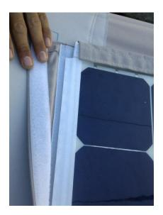
Note that the Velcro is both sewn and glued to the panel. Also note that in this case a bit more clearance could have been left between the Velcro and the cells to avoid shading the cells.
