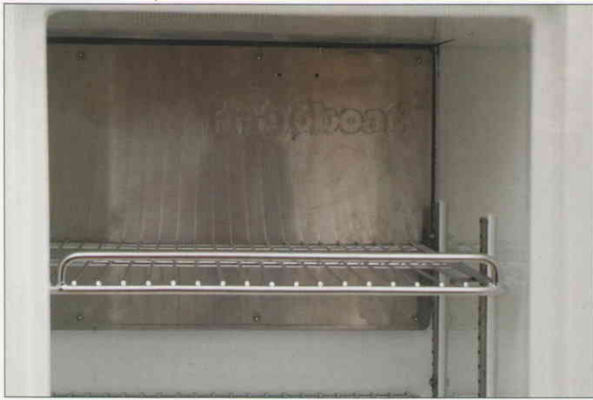
The refrigerator/freezer setup on the author's own boat. Left —The flat-plate evaporator in the icebox, shown here, takes up less space, and weighs less, than a holding plate, but requires a constant-cycling refrigeration unit. In an evaporator plate, the evaporator coil consists of a series of passages formed between thin sheets of aluminum sandwiched together; there is no tank of fluid, so the evaporator plate is much smaller and lighter than a holding plate. The evaporator plate absorbs heat directly from the air in the icebox. Right —Details of the freezer: note the double seals on the lid, the flat-plate evaporator bent around three sides on the inside, and the ice tray held to the evaporator with bungee cords.
