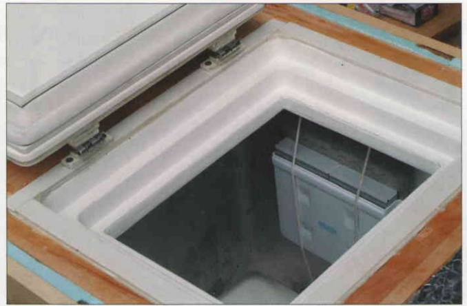
The refrigerator/freezer setup on the author's own boat. Left —The flat-plate evaporator in the icebox, shown here, takes up less space, and weighs less, than a holding plate, but requires a constant-cycling refrigeration unit. In an evaporator plate, the evaporator coil consists of a series of passages formed between thin sheets of aluminum sandwiched together; there is no tank of fluid, so the evaporator plate is much smaller and lighter than a holding plate. The evaporator plate absorbs heat directly from the air in the icebox. Right —Details of the freezer: note the double seals on the lid, the flat-plate evaporator bent around three sides on the inside, and the ice tray held to the evaporator with bungee cords.
