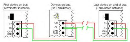
The control at each end of the bus must have a terminator installed. The terminator is a two pin jumper located on the circuit board next to the CAN connector labeled CT. Place this jumper only on the first and last control in your system.
