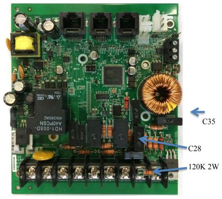
Remove C35 and C28 for contactor or pump relay connected to fan output. Install a 120K 2W resistor on fan L1, L2.
