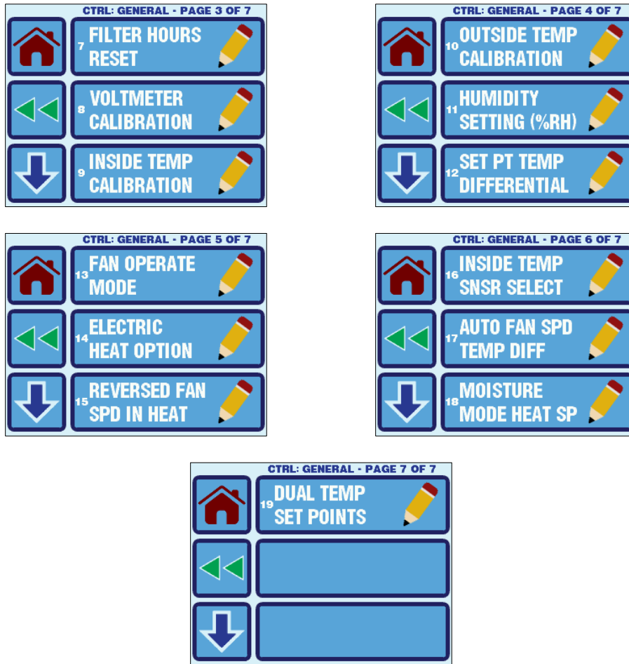
Figure 18 – EasyTouch General Settings Menu Screens for Standard DX/CW System
