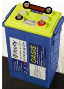
The battery will be shipped with the connection bar shown above. This connects the 2 cells inside the module in series making the battery 4V and 450Ah. For a 12V x 450Ah bank, connect 3 x 4V/450Ah in series (3S). For 24V x 450Ah, connect 6 in series (6S). For 900Ah x 12V, it must be 3S x 2P (3 batteries in series and then parallels with the other series string). For 900Ah x 24V, it must 6S x 2P
