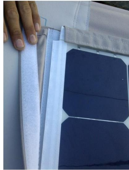
Note that the Velcro is both sewn and glued to the panel. Also note that in this case a bit more clearance could have been left between the Velcro and the cells to avoid shading the cells.
