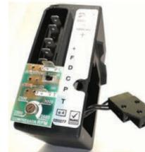
3. **Merlin Smart Speed Controller:** Mounts on compressor controller. Speed adjusted automatically dependent on thermostat cycle timing. Ramp-up start sequence for protection of electronics. LED shows compressor speed or compressor idle status.
