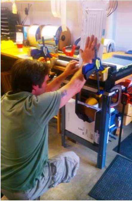
1: Glenn uses a bending machine to hold the evaporator in place while he bends up.
